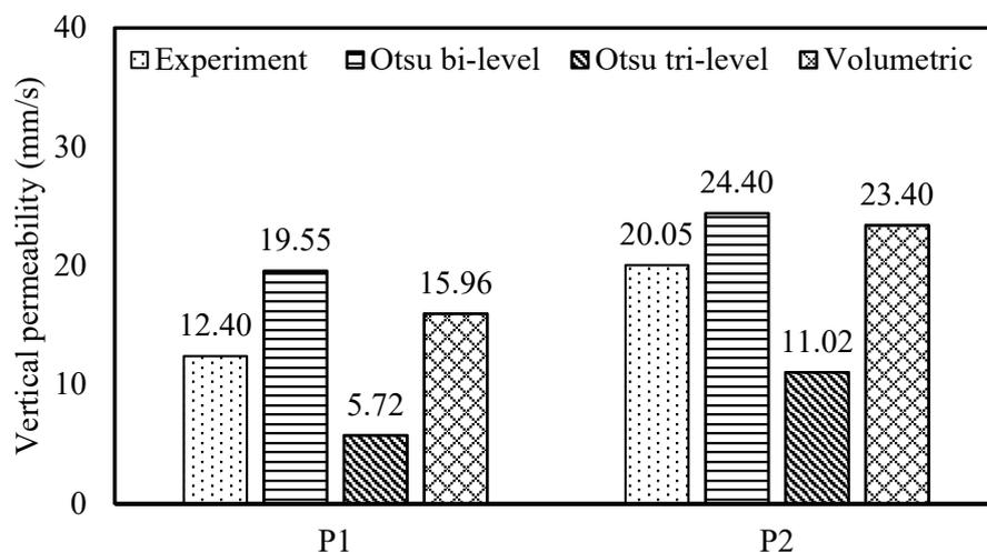
**Fig.6: Vertical permeability results of thresholding techniques**
