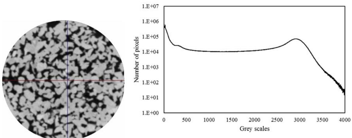
**Fig.2: 2D sliced raw image of pervious concrete and its grey scale histogram**
