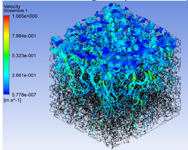
**Fig.10: Velocity streamlines of pervious concrete sample**
