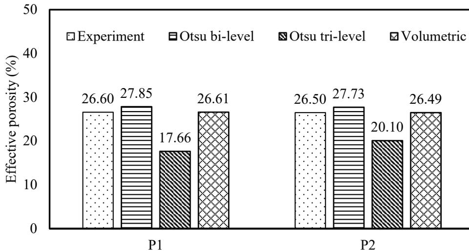
**Fig.11: Influence of thresholding techniques on effective porosity (%)**
