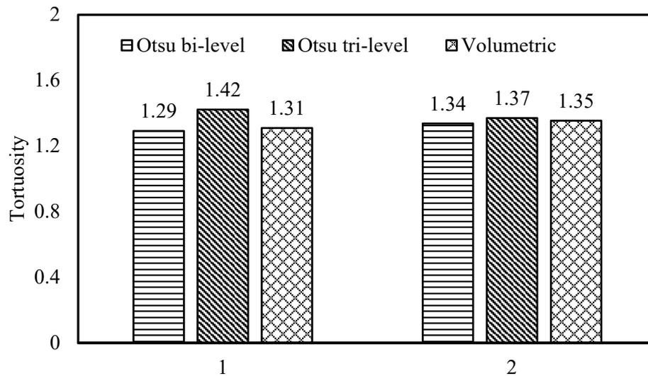
**Fig.9: Influence of thresholding techniques on tortuosity**
