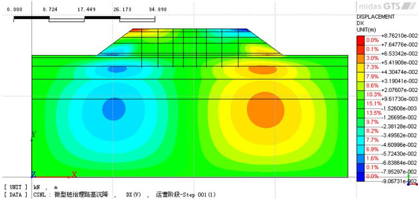
**Figure 4 Horizontal displacement during operation**
