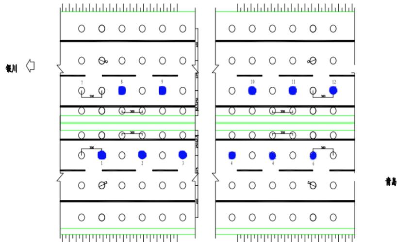
**Figure.1 Schematic layout of K557+345 earth pressure box**
