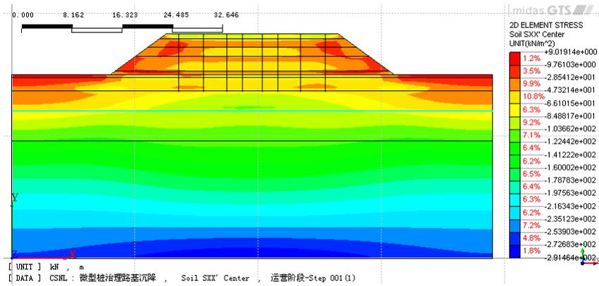
**Figure 3 Horizontal stress during operation**
