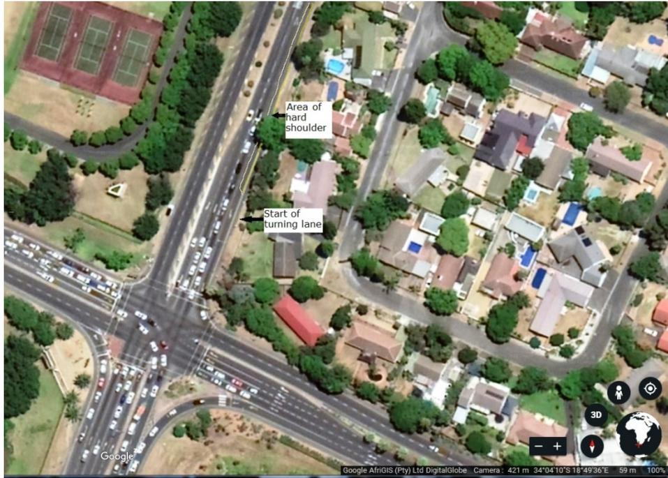
**Figure 1: Typical road layout showing hard shoulder and turning lane (this example taken from Site 2), Google Earth 2019.**
