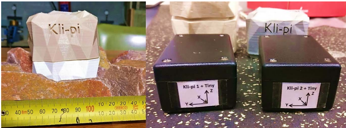
Figure 1: Kli-Pi 3D printed shell / exoskeleton and the internal IMU box containing all the electronics
