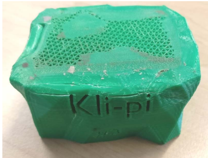
Figure 2: Unfinished shell print illustrating the geometry and internal structure
