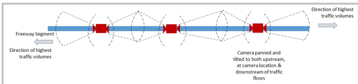
**Figure 6: Roaming view camera surveillance**
