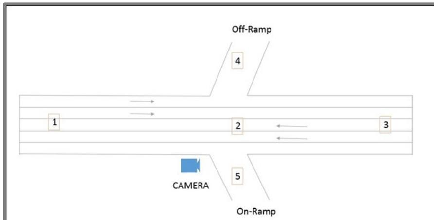
**Figure 9: Setting up pre-sets at an interchange**
