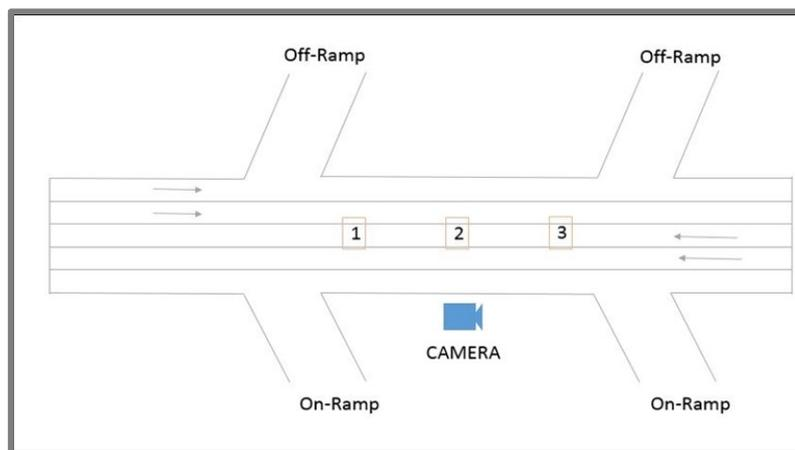
**Figure 8: Setting up of pre-sets on freeway segments**
